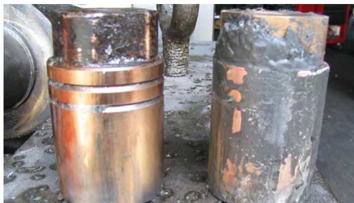
Comparison of Chem-Trend plunger lube tip (left) and the competitive product tip (right). Both tips have run for 2500 shots.
