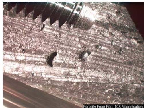
Fig 2: Shrinkage porosity
