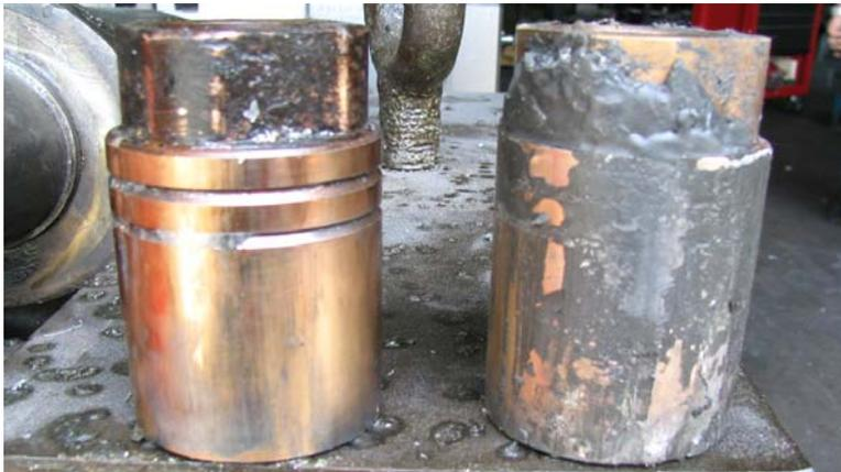
Fig 8: Comparison of Chem-Trend plunger lube tip (left) and the competitive product tip (right).
